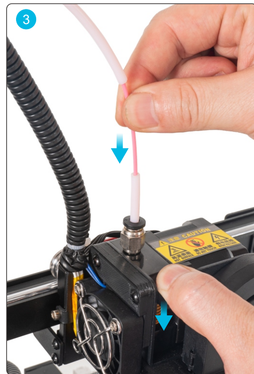
Press down on the elastic buckle of the extruder and insert the filament to the bottom of the print head 向下按压挤出机的弹力扣, 将耗材插到打印头底部
