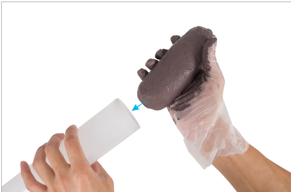
Put the clay into the barrel 将泥团放入料筒里
