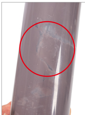
Bubbles were found after filling the mud
