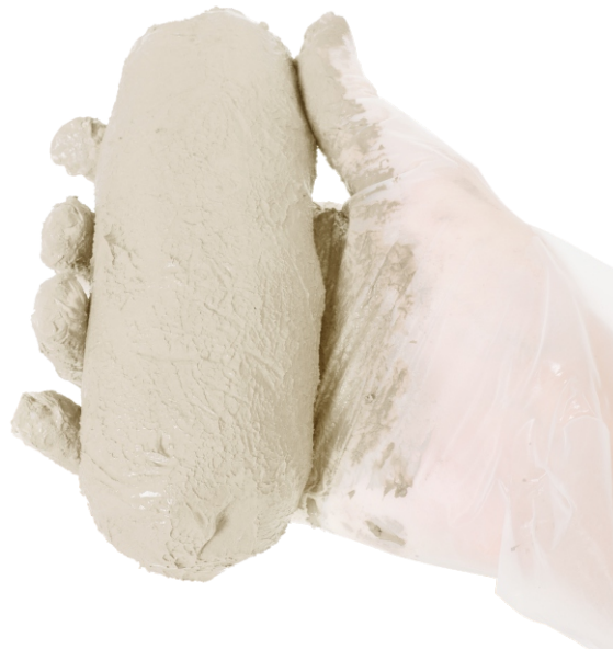
Knead the dough into a cylindrical shape slightly smaller than the material barrel 将泥团揉成比料筒略小的圆柱形
