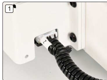
Insert the right Z-motor line 插入右边Z电机线
