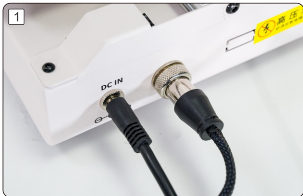
Insert the power cord and motor connection cable 插入电源线和电机连接线
